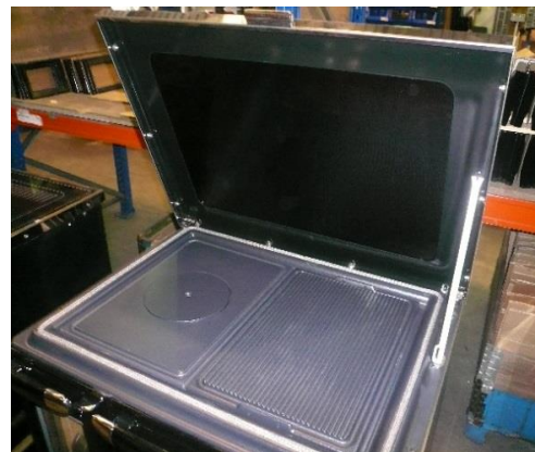
Figure No.28 - Protective supports beneath glass-ceramic top surface
